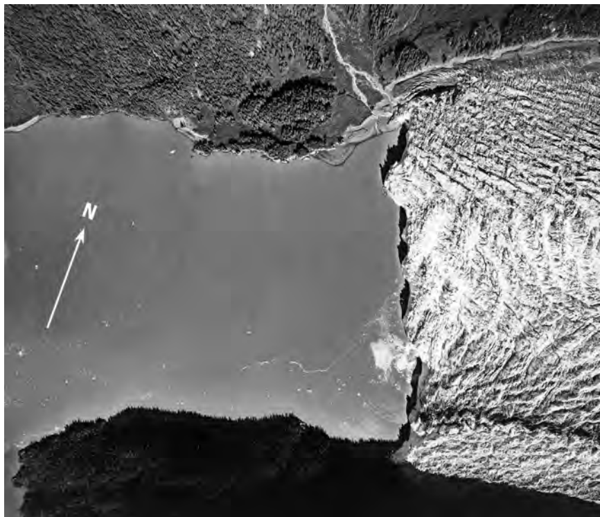
Figure 253. —17 August 1999 vertical aerial photograph of the terminus of Meares Glacier. Before the date of the photograph, Meares Glacier advanced into Ranney Creek (to the left of the terminus), diverting its waters to the south. Subsequent calving and retreat of the ice at the western margin resulted in the stranding of a block of ice along the edge of Ranney Creek. Subsequently, the ice was incorporated into the advancing terminus of the glacier. Photograph no. R3-FL7-FR119 from the U.S. Bureau of Land Management.
